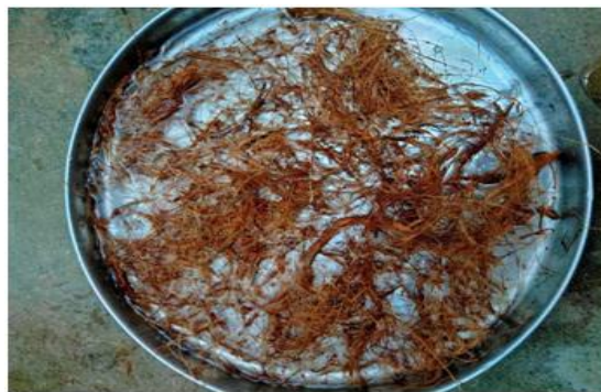
Figure 6: - Coconut coir fibres soaked in NaOH solution
