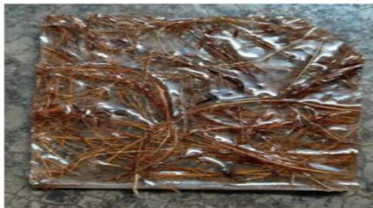
Figure 10: - Sample Plate of Coconut Coir and Lapox of 35mm x 35mm
