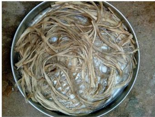
Figure 5: - Jute fibre soaked in NaOH solution
