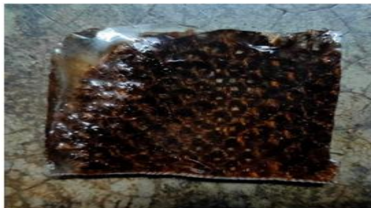
Figure 9: - Sample Plate of Jute Fibre and Lapox of 35mm x 35mm
