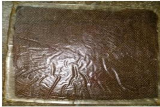
Figure 7: - Sample Plate of Jute and Lapox
