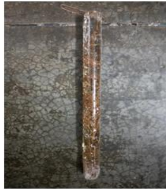
Figure 11: - Cylindrical sample of Coconut Coir and Lapox
