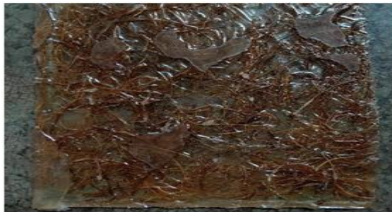
Figure 8: - Sample Plate of Coconut Coir and Lapox
